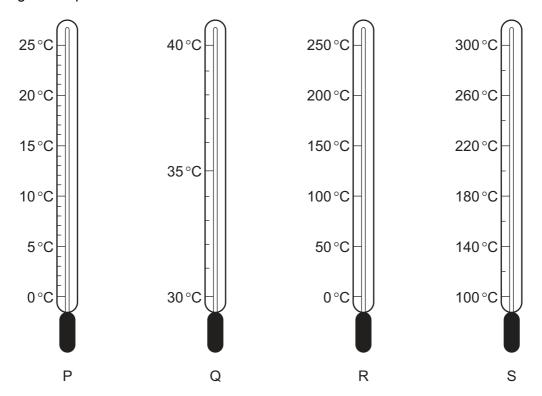
Which thermometer has the greatest sensitivity and which thermometer has the greatest range?
