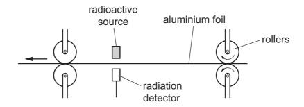
What is the most suitable radioactive source for the system?
